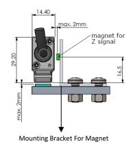
The magnet and Z reference sensor must be parallel to each other for the external Z reference signal.
